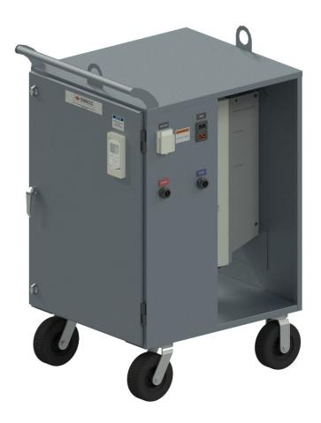
The ALT-P series power carts are built to take a standard single phase 240 Volt generator and allow you to run a three phase pump motor up to 20 hp or rating of the generator and cart. This cart is built to run one pump, bypassing the pump control station all together. Providing extended running capability after severe storms and power failures.
